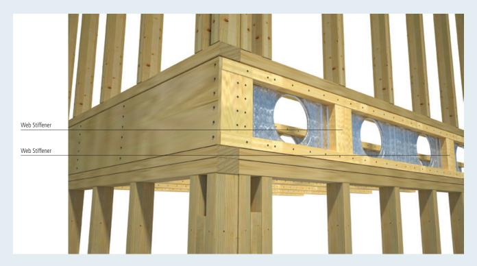
Note: If a web hole occurs over the support, add a pair of web stiffeners as close to the support as possible but covering the steel web sufficiently to fix the minimum nailing required through the web.
