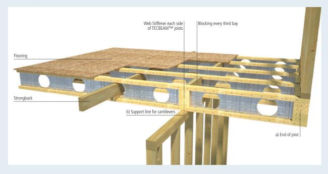
c) at the supporting walls, beams, posts, in continuous spans
