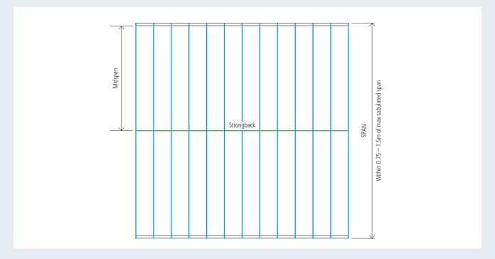
• Where the joist span is over 6m or within 0.75m of the tabulated span, install two rows of strongbacks; placed approximately at one third points of the joist span.
