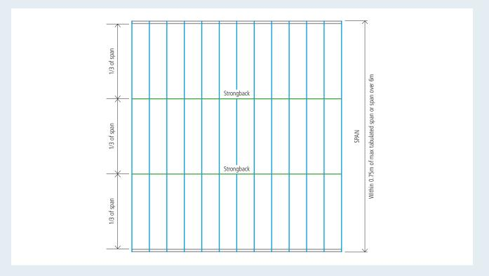
• For continuous spans – add a Strongback in the shorter span even if it is less than the spans indicated above.
