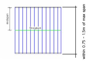
• Where the joist span is over 6m or within 0.75m of the tabulated span, install two rows of strongbacks, placed at approximately the one third points of the joist span
