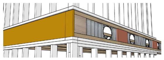
Note: If a web hole occurs over the support, add a pair of web stiffeners as close to the support as possible but covering the steel web sufficiently to fix the minimum nailing required through the web.
