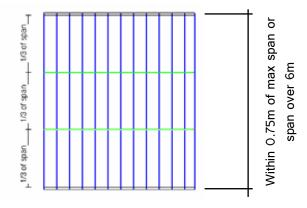
• For continuous spans - add a Strongback in the shorter span even if it is less than the spans indicated above.
