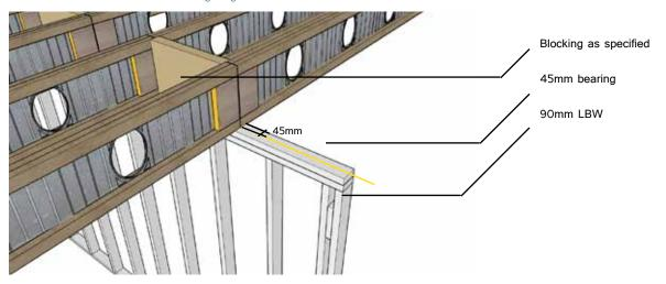
Alternately, Tecbeam joists can be staggered at internal load bearing walls for full 90mm bearing
