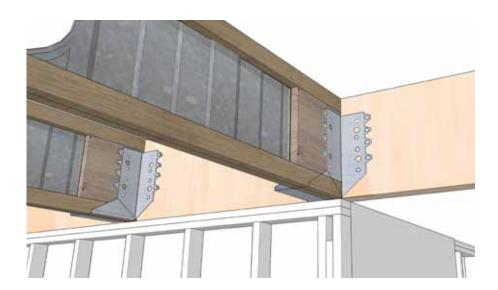
• Where TECBEAM joists carry higher loads e.g. double joist at stair void, a combination of a joist hanger on one joist and a steel angle bracket fixed with 2M12 bolts on the other joist can be used. See detail below and refer to Tecbeam Standard Details.
